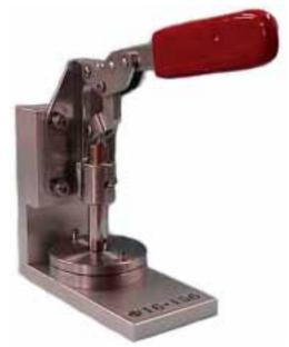
It is a punching tool for the hyperactive lithium metal used as a cathode. It has a plastic die in order to avoid fire.
